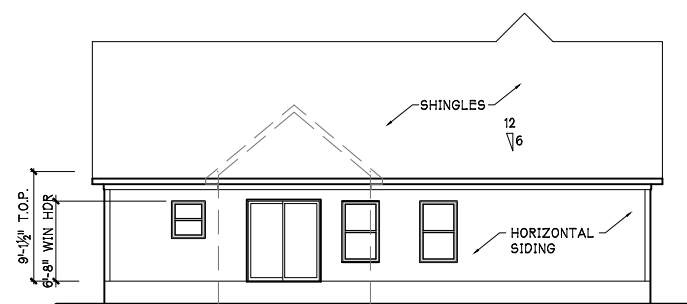
4 REAR ELEVATION SCALE: 1/16"=1'-0" (11"x17" SHEET SIZE) SCALE: 1/8"=1'-0" (22"x36" SHEET SIZE)
